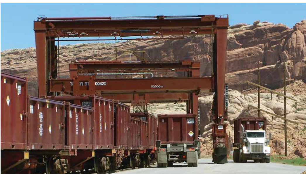
Top: Once featured on a postcard, the Uranium Reduction Corporation mill began processing ore on October 1, 1956. [Image courtesy Moab Museum] Bottom: A powerful gantry crane is used to lift containers full of contaminated material from trucks, and place them on a train that delivers the load to Crescent Junction. [Photo courtesy Dept. of Energy / Moab Sun News file photo]
